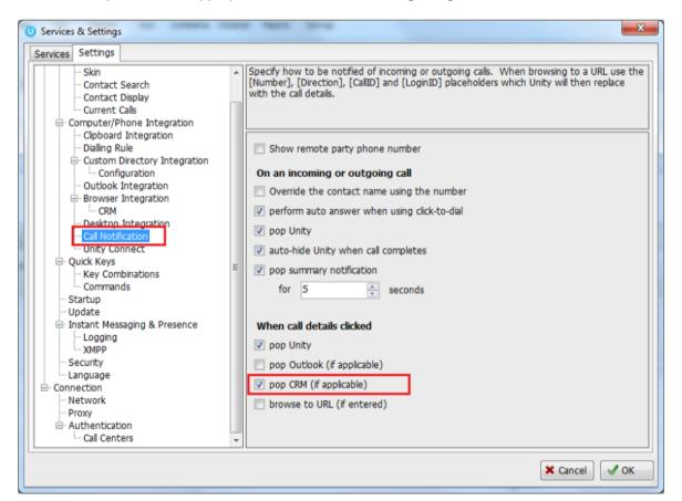
Unity can also be configured to automatically pop the CRM contact when the call isanswered, which depends on the Automatic Contact Pop tab settings as shown below.
